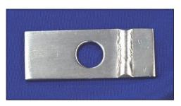
Welded coupons can be prepared with or without the use of filler metal. The autogenous weld is prepared without the use of filler metal. This type of weld is the most economical method. Autogenous welds are commonly used to evaluate corrosion rates of welded materials and the usage of these materials in corrosive environments. An autogenous weld is produced by GTAW and can be used to test material weldability and gas shield usage, and to set welding parameters.
