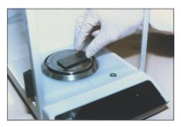
Metal Samples offers post exposure coupon analysis. Our trained technicians will perform weight loss analysis and determine mils per year (MPY) corrosion rates of your exposed test samples. We are in adherence to ASTM-G1 specifications for cleaning and analyzing coupons.
